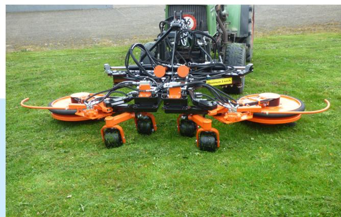
The Duo-Swing models are also available for mounting in the front linkage of the tractor for an optimal view of the two discs.
