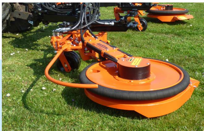
To reduce the risk of damage to young trees and to be able to work on slopes, the swing arm can be equipped with a hydraulic feeler bar.
