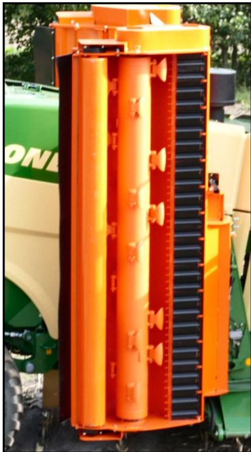
Standard 2.2 kg heavy flails. Less sensitive to stones. Mounted with 20mm bolts and replaceable wear bushes in the mounting ears.
