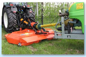
Tmodels can be equipped with a unique "Perfect" mow-spray frame that has been designed so that both the front and the rear of the mower is able to move freely from the headstock.
