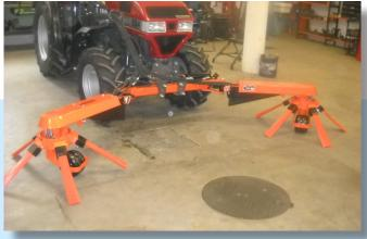
The SPD models are equipped with a carriage beam for fix mounting to the front of a tractor.
