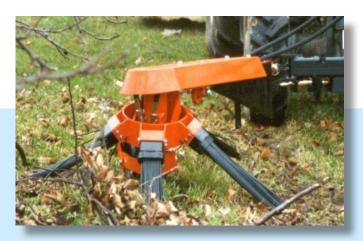
The sweeper head position is adjustable both in working angle and in working height, which assures a high quality working result in all conditions.
