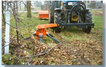
The SPF front mounted models are equipped with a carriage beam for fix mounting to the front of a tractor. A headstock for attachment to the tractor 3-pt front linkage is optionally available.
