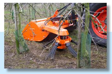
The sweeper head position is adjustable both in working angle and in working height, which assures a high quality working result in all conditions. For perfect terrain adjustment the sweeper head is supported by a swivel wheel.
