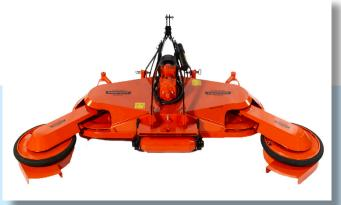
Swing arms are spring loaded and can be set in different positions to vary the cutting width. At the finest touch of the tree the rubber covered swing arm wheel rotates and deflects its cutting blade away from the tree.
