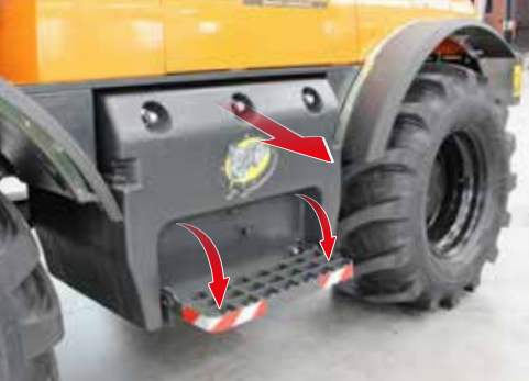
Zavorra mobile con gradino Moving ballast with step
