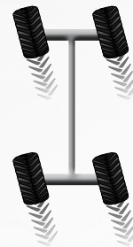
4 RUOTE STERZANTI PARALLELE 4 PARALLEL STEERING WHEELS
