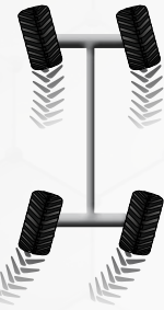
4 RUOTE STERZANTI PARALLELE 4 PARALLEL STEERING WHEELS
