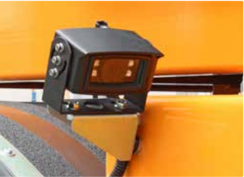
Telecamera retromarcia Reverse gear camera
